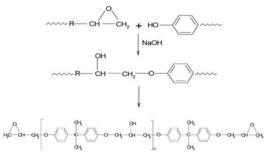
Curing of epoxy resins takes place either through epoxy group or hydroxyl group involves two types of curing agents, catalytic system and polyfunctional cross-linking agents. The catalytic cross-linking occurs in presence of hydroxyl group, which may be present due to the following circumstances:
