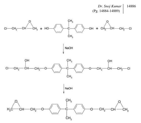
If diglycidyl ether is considered as a diepoxide; it will further react with hydroxyl groups to form high molecular weight epoxy resin as shown below-
